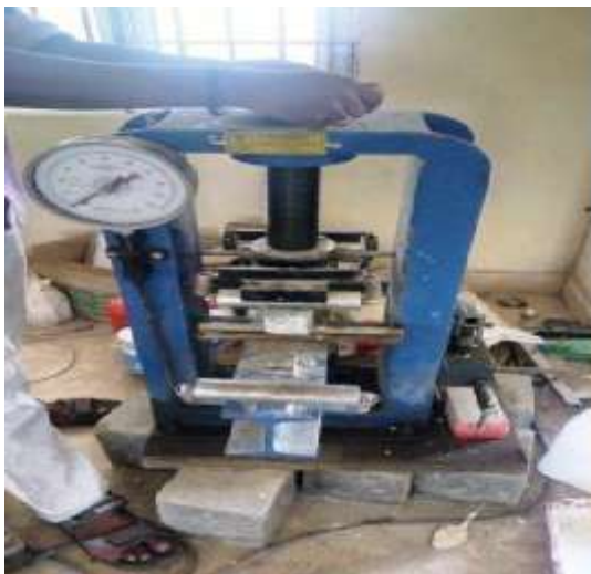
Fig. 3.5 FRACTURE TEST SPECIMEN LOADING
