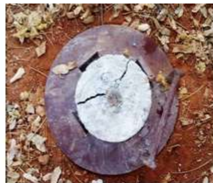
Fig. 3.12 IMPACT STRENGTH TEST SPECIMEN
