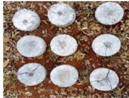
Fig. 3.11 IMPACT TEST SPECIMEN
