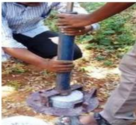
Fig. 3.10 IMPACT STRENGTH TEST LOADING
