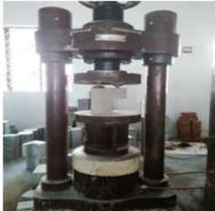
Fig. 3.9 SHEAR STRENGTH TEST LOADING
