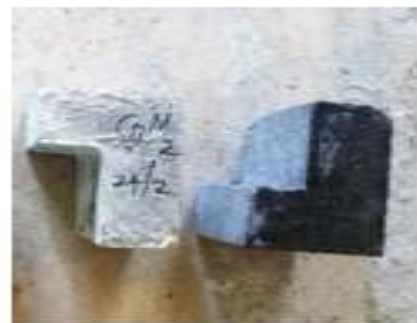
Fig. 3.8 SHEAR STRENGTH TEST SPECIMEN
